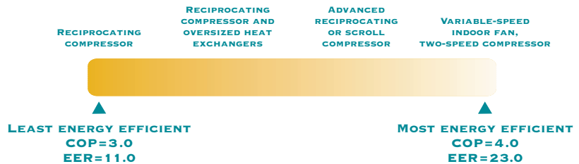
FIGURE 23. OPEN SYSTEM EARTH ENERGY SYSTEM EFFICIENCY (AT AN ENTERING WATER TEMPERATURE OF 10°C)
